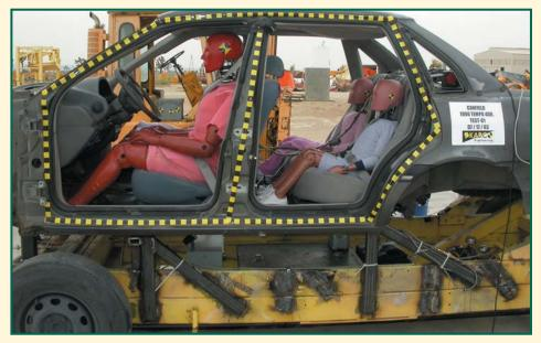
Plaintiff's sled testing – pre-impact (above). Testing showing failure of driver's seatback in 1990 Ford Tempo (below).
