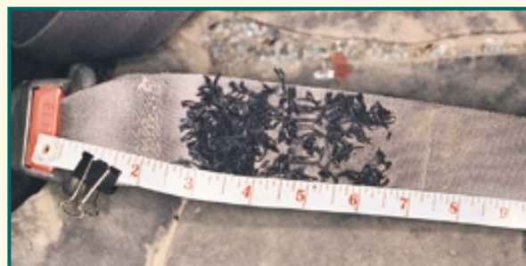
Failed seat belt.
