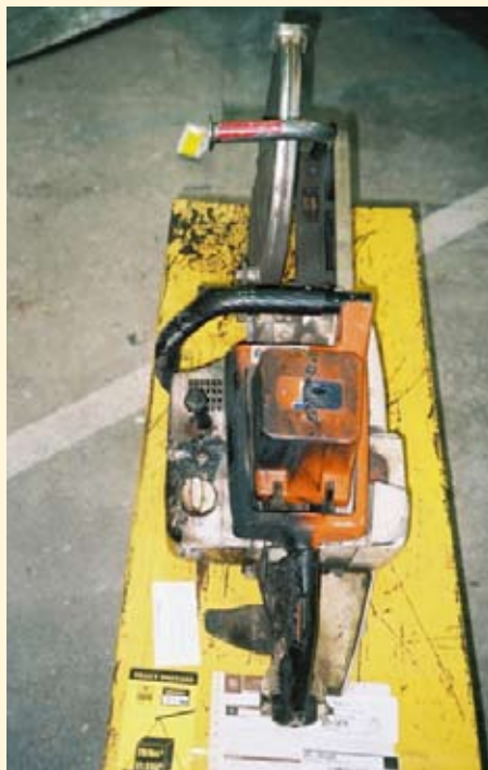
A cutsaw caught fire when fuel contacted rail heated from welding and caused substantial burns to a railroad employee.
