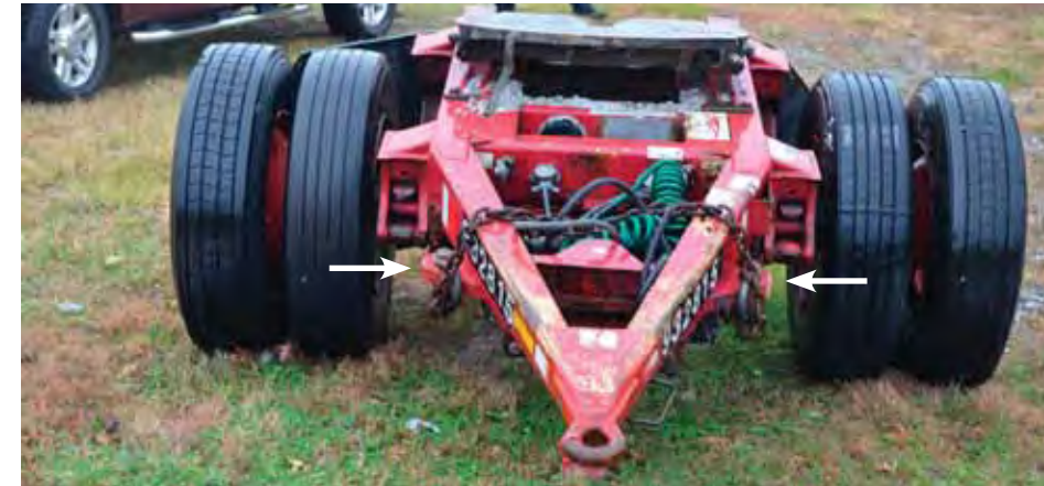
Failure to properly use safety chains, which are indicated next to the white arrows, allowed a rear trailer to detach and cause a truck driver to drive into an embankment.
